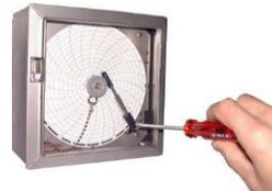
Zero Adjustment: turn the plastic screw Gently. At normal usage zero adjustment is not required.
