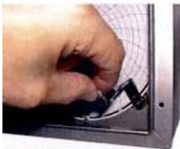
Remove the protective cover from the recorder pen.
