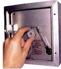
Open the recorder door and remove the knob of the clockwork by turning it clockwise.
