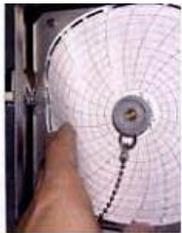
Ensure that the chart is placed under the 4 chart clips on the lower panel.
