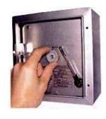
Open the recorder door and remove the knob of the clockwork by turning it clockwise.
