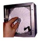
Return the knob of the clockwork by turning it anti-clockwise. **Wind up max. 5 turns!!**
