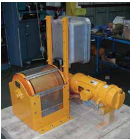
Explosion proof motors and controls
