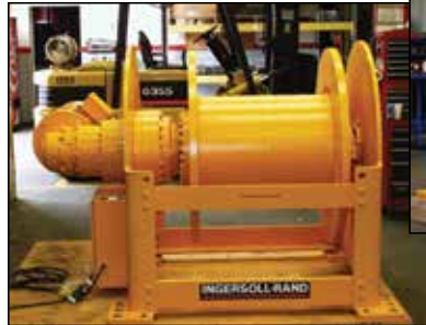
50,000 pound hose positioning winch
