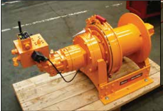
16,400 pound hydraulic pipe handling winch
