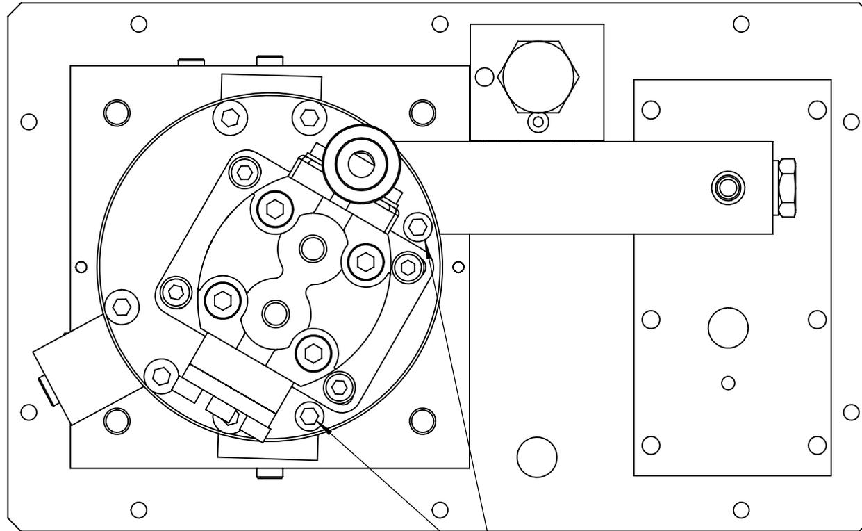
REMOVE THE TWO CURRENT SCREWS FROM THESE TWO POSITIONS AND REPLACE WITH ITEM NO. 10 (FAS008SP080)
