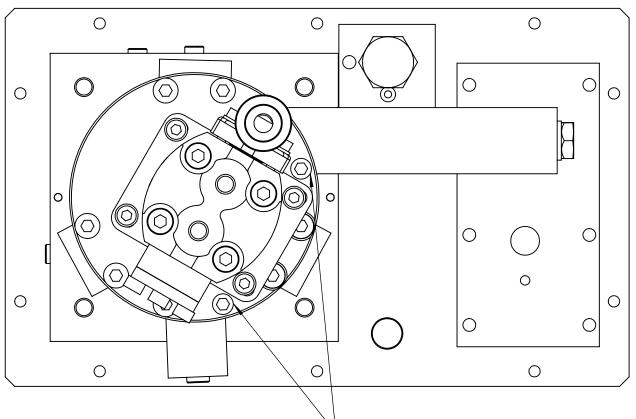
REMOVE THE TWO CURRENT SCREWS FROM THESE TWO POSITIONS AND REPLACE WITH ITEM NO. 10 (FAS008SP080)
