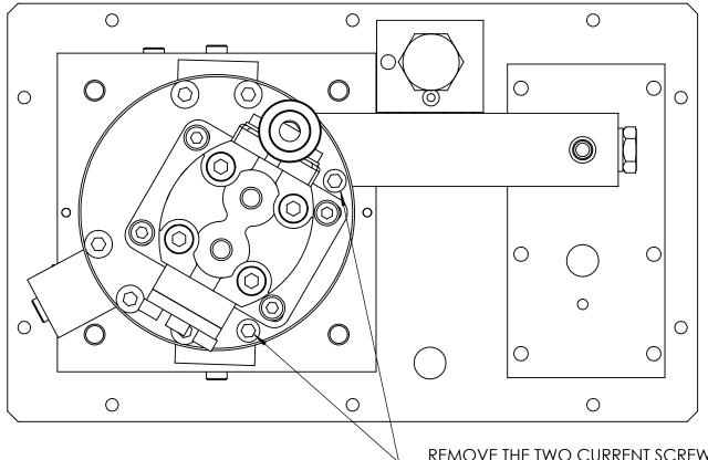
REMOVE THE TWO CURRENT SCREWS FROM THESE TWO POSITIONS AND REPLACE WITH ITEM NO. 10 (FAS008SP080)
