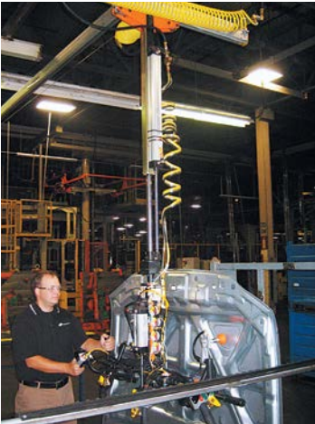
Torque tube with integrated vacuum handling device
