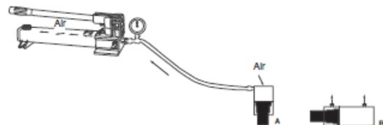
Single Acting Cylinders: Position the cylinder below the level of the hydraulic pump with the piston of the cylinder pointed downwards (as in A, in the diagram above.) Fully extend and retract the piston
