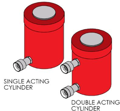
Connect the hoses between the cylinder and the pump ensuring that the coupling/s are fully **hand tightened** only. **Never** use wrenches to attempt to connect the coupling/s, incorrectly connected coupling/s is one of the most common causes of faulty operation.
