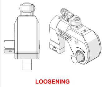
Figure 5.5: Direction of Rotation of the Square Drive
