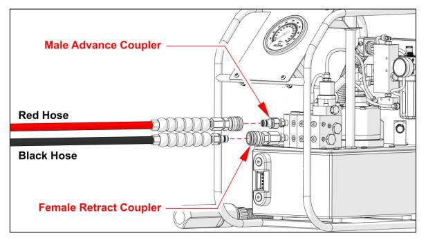
Figure 5.3: Connecting to the Pump
