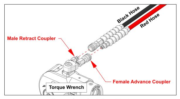
Figure 5.4: Connecting the Torque Wrench
