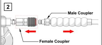
Figure 5.2: Hydraulic Disconnections
