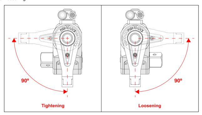
Figure 5.7: Correct Reaction Arm Quadrants
