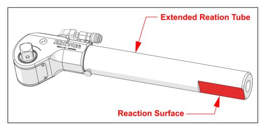
Figure 5.8: Extended Reaction Arm Orientation & Reaction Surface
