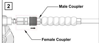
Figure 5.1: Hydraulic Connections
