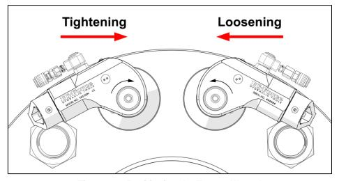
Figure 6.1: Positioning the Torque Wrench
