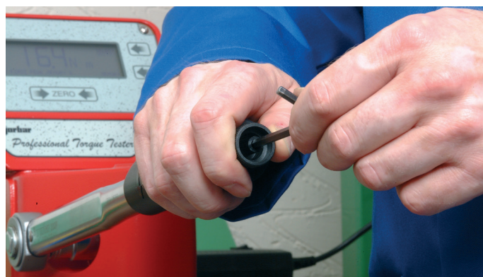
Setting a 'P' Type Torque Wrench
