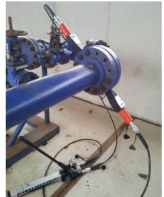
Ensure that the wedge step is inserted as far as possible into the components to be separated. **Do not** hammer the tool into a gap which is too small.
