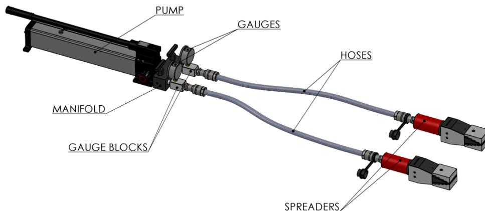
**Note:** A loose coupler will slow or stop the oil flow and is the most common cause of faulty operation.
