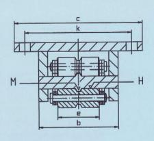
MOd. AM-H (H = hardened and machined centre plate), AM-H-50CrV4 (roller material 50CrV4)
