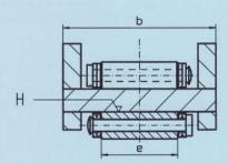
Mod. C, C-H (H = hardened and machined centre plate), C-H-50CrV4 (roller material 50CrV4)
